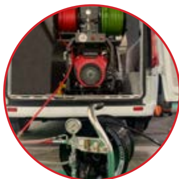
domestic drains and condominial sewer cleaning units
