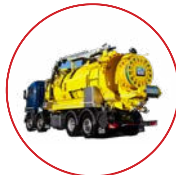
Vehicles equipped for water jetting
