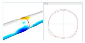
Our main-sewer inspection cameras have other features too: Equipped with an optionally available scanning function, they detect even the smallest deformations in main lines using 2-point precision lasers and measure them precisely both point by point and across the entire reach. Due to the 3D display of the pipe, deformations can be determined accurately.
