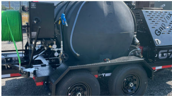
Water system controls mounted near control box and jetter reel for user-friendly layout.
