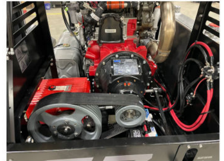
An enclosed engine compartment gives this jetter a clean look with user-friendly access for engine and water pump maintenance.
